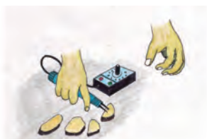
Moisture content testing
